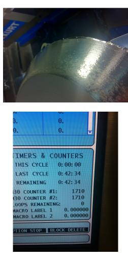
This cover still has finish passes to clean up the surface of the cover aswell as actual design into the face.
