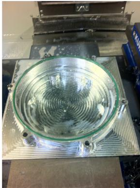
Jaws are machined to flip the entire cover over and machine the other side
