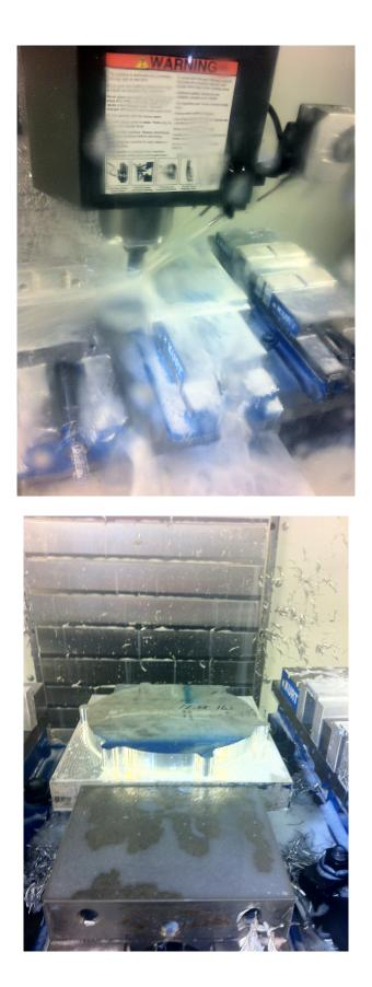
Now the inside is cleared in multiple steps, holes are drilled, and o-ring groove is machined.
