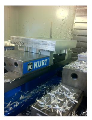
A 42 minute program is ran to machine in full 3D the entire outer profile, in production this will be done in a lathe for optimum finish, but 42 minutes saves from the need of another machine being setup.
