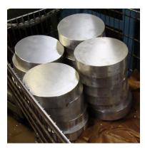
Then we turn the billet blanks down on our CNC lathe
