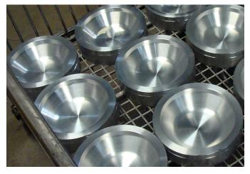
We then flip over the blanks and turn down the face on our CNC lathe
