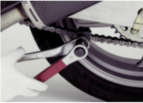
**4a.** Use a 27mm closed in wrench to hold firm the body of your chain tool while using a closed end 19mm wrench on the tool's hexagon bolt head to tighten. It will be easier to tighten the bolt if you position your wrenches 30° apart.
