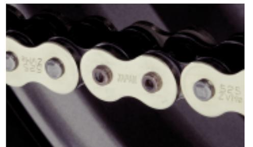
**12a.** After pressing the sideplate on, disassemble the chain tool and remove it from the chain. The next step is to flare out the pins heads for ZJ (Rivet type) or installing the slide clip for the FJ (Cliptype) master link.
