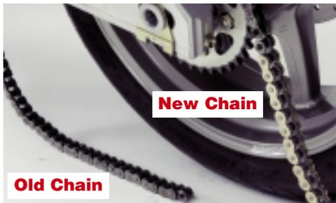
**7a.** Connect the new chain to the old chain using either a wire or connecting link. Shift transmission into neutral and slowly pull the old chain from under the swingarm toward the rear which then pulls the new chain from the top towards the countershaft sprocket. When new chain goes completely around the front sprocket and out under the swingarm, disconnect the old chain and pull both ends together under the center of the swingarm.
