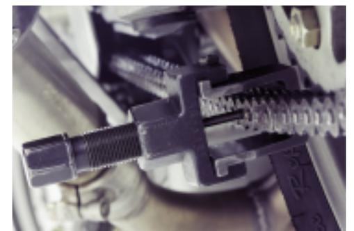
**3a.** To align the tool's Cutting pin with the chosen pin head, turn the tool's large bolt head clockwise "by hand" until the Cutting pin comes in contact with the pin head. At this point, make sure that the cutting pin is lined up with the center of the pin you wish to push out.
