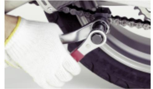
**15a.** Hold the hexagon part of the tool body by with a 27mm closed in wrench, and the bolt head with a 19mm closed end wrench; turn clockwise until the flare part of the pin head makes contact with the surface of the side plate.
