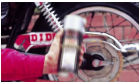
**6a.** Shake the chain lube can a couple of times to mix up the ingredients.
