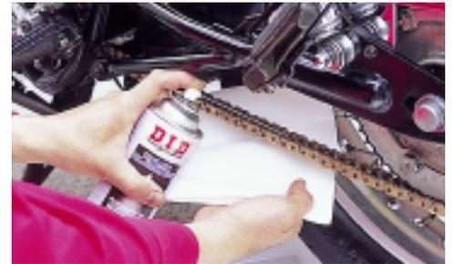
**2a.** Before applying chain cleaner, put a tray under the chain and hold a towel behind the chain to prevent overspraying. Put the motorcycle on stand to allow rotating the rear wheel. Spray on cleaner while rotating rear wheel by hand to clean the entire chain.
