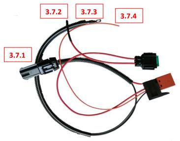
3.7.1 Take the actuator and insert the 2 **Red** wires (no matter the order) into the Male Superseal connector provided.
