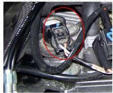
Unplug connectors and put in the between the IRC harness with the bypasses labelled with a number (1, 2, 3 and 4. Looking the engine from backwards, disconnect the leftwards coil connector and put the upkit bypass number "1" between it and the coil.
