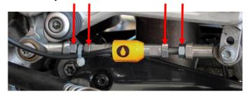
Install sensor and rod with uniball links on both ends, most bikes have uniballs stock, check that the shiftrod does not rub or touch anything. Put sensor far from very hot parts. Make sure wire has a slight bend/loop so it does not tighten up and pull at the sensor during up or down shift. Warranty doesn't cover ripped out wires.
