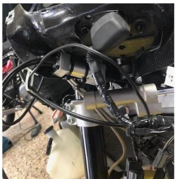
Wire movement inside its sheath must freely move. Connect the cable from twistgrip to throttle pulley, adjust the free play as in std bikes. Adjust the eventual return cable too. Anything must work as in std bike.
