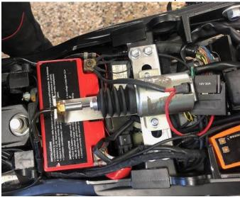
VA universal cable is provided in the kit. Cut it according to your needs with registers in the middle in order to have enough adjustment travel
