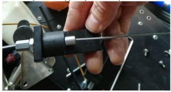
Put the piston against the cylinder cover on throttle side. Fix the locking pin against the piston, close the covers and fix the blipper cylinder body in position.
