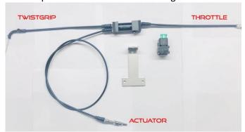
Cable from twistgrip to throttle, pass trough freely while the actuator is connected to it and acts only on demand.
