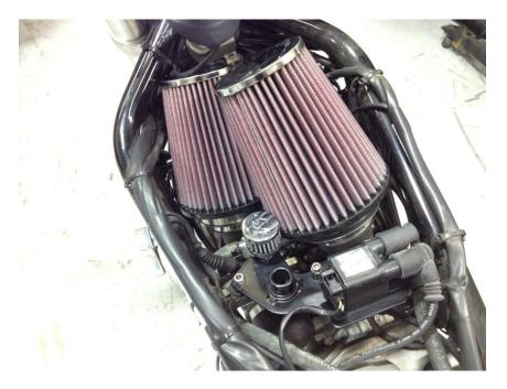
19. Install the crank case breather filter.
