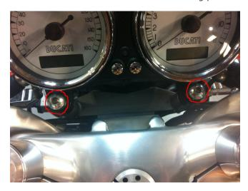
Install the supplied mounts as pictured below with the supplied button head bolts:
