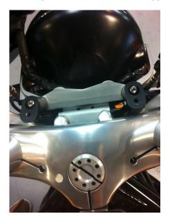
Using the factory bolts mount the gauges onto the brackets. Tolerances vary on the headlight location, if the gauge contacts the headlight use a washer to space the gauges up to avoid contact with the headlight.
