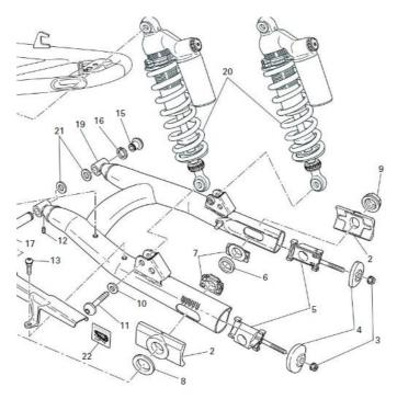
Install: remove rear wheel and components: 2, 3, 4, & 7 from the swingarm. Leave item 5 still in the swingarm. Locate both of item 3 (nut) and double nut the stud on item 5 in the swingarm, using the first nut to jam the second nut will allow you to remove the stud from the factory slider block. Repeat on the other slider block. With both studs removed remove old thread lock from the threads, reapply thread lock and torque to 22Nm.
