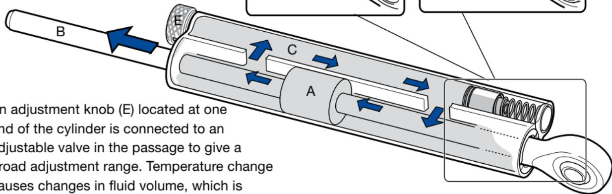
An adjustment knob (E) located at one end of the cylinder is connected to an adjustable valve in the passage to give a broad adjustment range. Temperature change causes changes in fluid volume, which is controlled by a pressurized reservoir (F) located at the other end of the steering damper. The fluid is pressurized either by a compressed closed cell rubber foam (Fig 1), or by a spring preloaded dividing piston (Fig 2).
